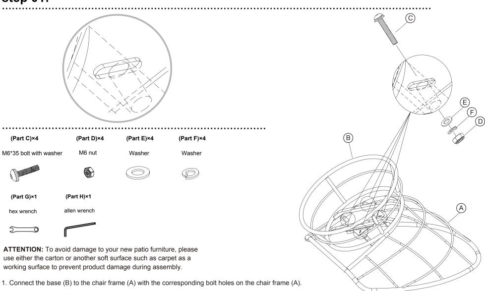
2. Secure with M6\*35mm bolt with washer (C), M6 nut (D), Washer (E) and Washer (F) by using hex wrench (G) and allen wrench (H).
