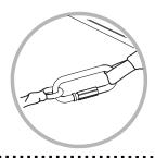
1. Open the hook of safety rope on the seat frame (E), pass through the iron loop on the lower hanging bar (C). Then tighten the hook of safety rope.
