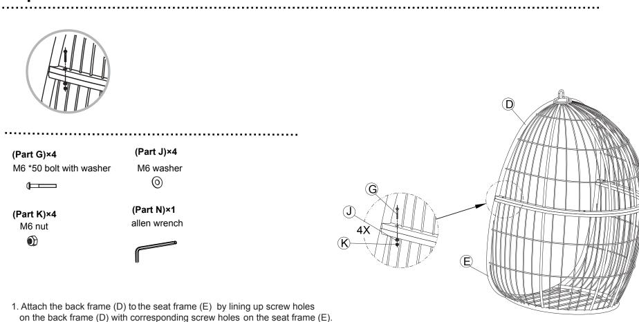
2. Secure with M6\*50 bolt with washer (G), M6 washer (J) and M6 nut (K). tighten using allen wrench (N) and wrench (O).
