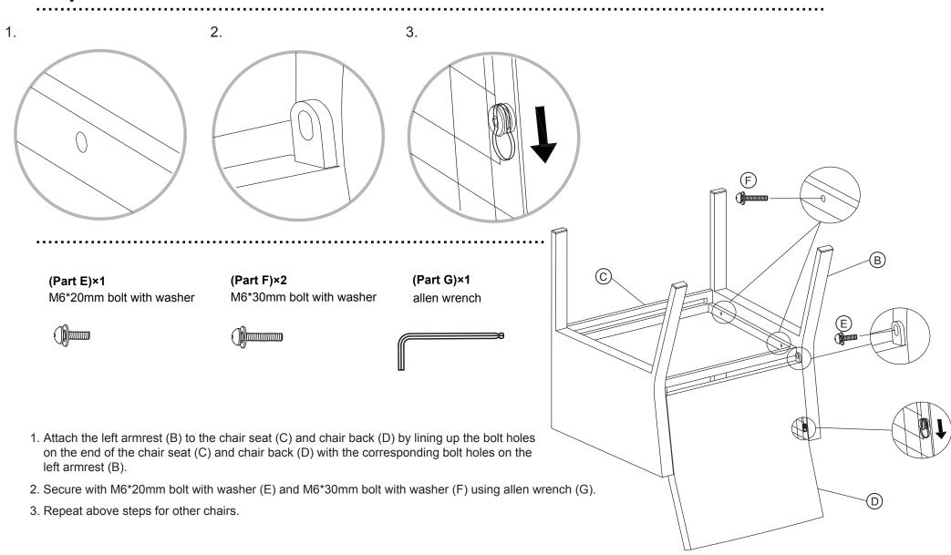
Do not completely tighten screws until all screws are in place.
