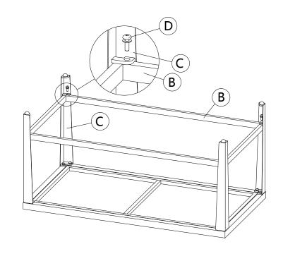
1. Attach the connector bracket (B) to the table leg (C) by lining up screw holes on connector bracket (B) with corresponding screw holes on the table leg (C). Secure with M6\*15 mm screw with washer (D), tighten using allen wrench (E). Repeat this step until another connector bracket (B) is secured to the table leg (C).
