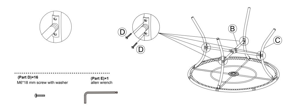
1. Attach the connector bracket (B) to the table leg (C) by lining up screw holes on connector bracket (B) with corresponding screw holes on the table leg (C). Secure with M6\*18 mm screw with washer (D), tighten using allen wrench (E). Repeat this step until another connector bracket (B) is secured to the table leg (C).
