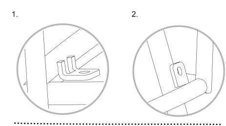
(Part C)×4 M6\*20mm bolt with washer (Part D)×1 allen wrench
