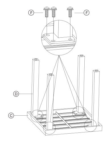
Do not completely tighten screws until all screws are in place.
