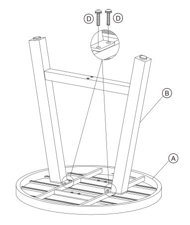
Do not completely tighten screws until all screws are in place.
