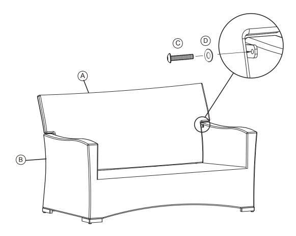
Do not completely tighten screws until all screws are in place.
