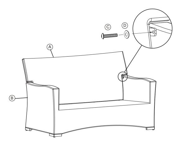
Do not completely tighten screws until all screws are in place.
