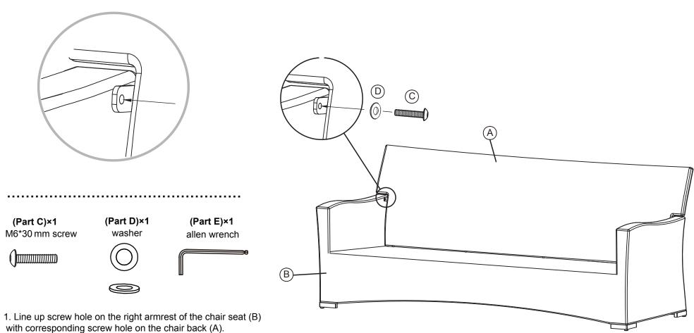
with corresponding screw hole on the chair back (A). 2. Secure with M6\*30mm screw (C) and washer (D) using allen wrench (E).
