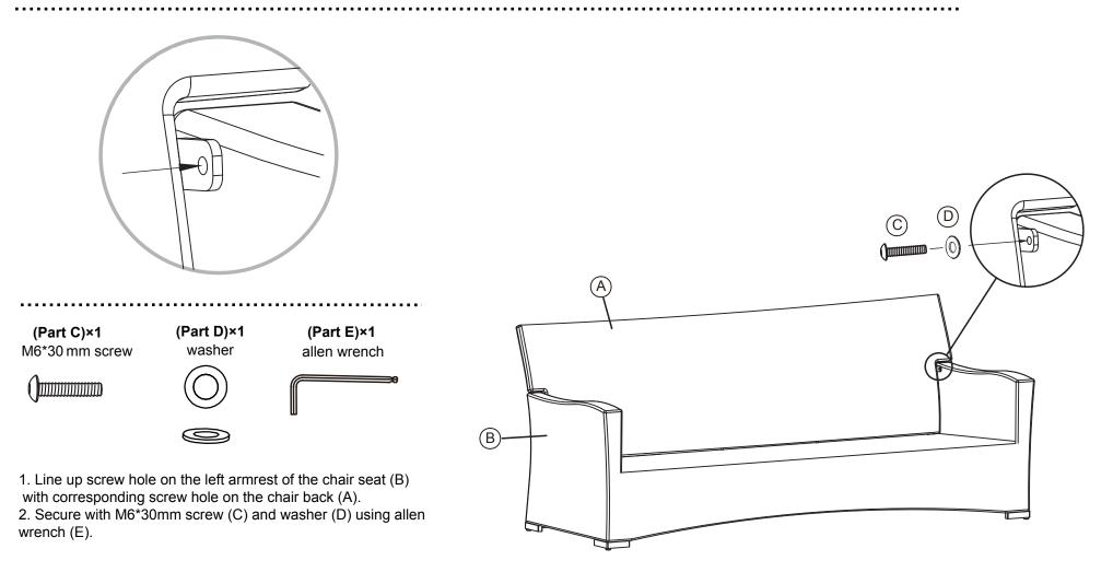
Do not completely tighten screws until all screws are in place.
