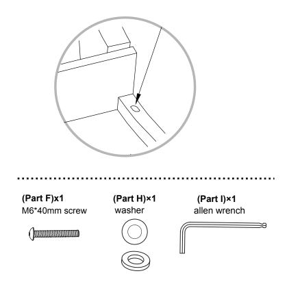
1. Secure with M6\*40mm screw (F) and washer (H) using allen wrench (I) on the left armrest (B) and back frame (C).
