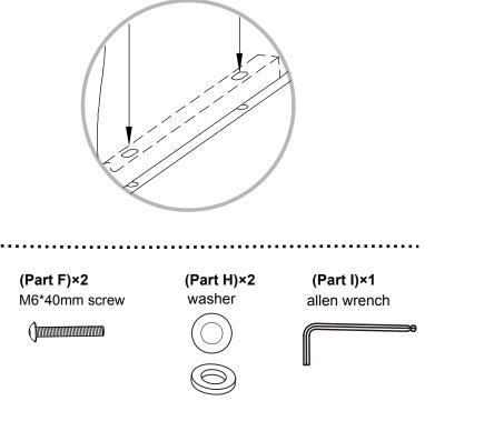
Attach the left armrest (B) to the seat frame (D) by lining up screw holes on the rleft armrest (B) with corresponding screw holes on the seat frame (D).
