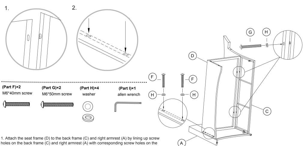
holes on the back frame (C) and right armrest (A) with corresponding screw holes on the back frame (C). 2. Secure with M6\*40mm screw (F) and washer (H) using allen wrench (I) on the right
