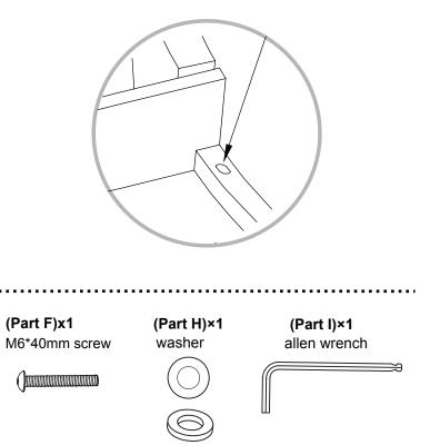
1. Secure with M6\*40mm screw (F) and washer (H) using allen wrench (I) on the left armrest (B) and back frame (C).
