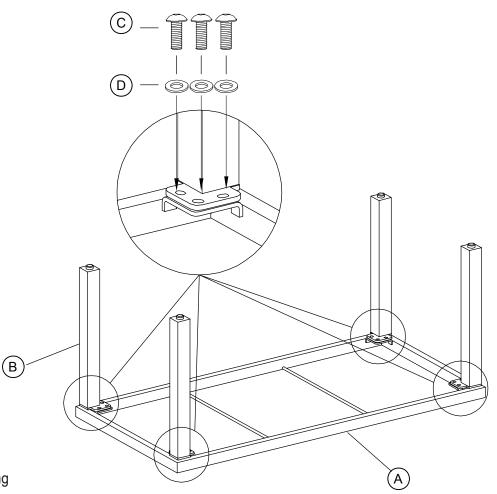
Do not completely tighten screws until all screws are in place.
