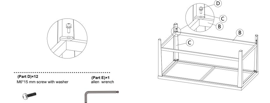
1. Attach the connector bracket (B) to the table leg (C) by lining up screw holes on connector bracket (B) with corresponding screw holes on the table leg (C). Secure with M6\*15 mm screw with washer (D), tighten using allen wrench (E). Repeat this step until another connerctor bracket (B) is secured to the table leg (C).
