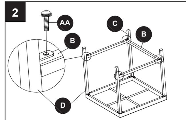
Once all connections are made, tighten AA with BB.
