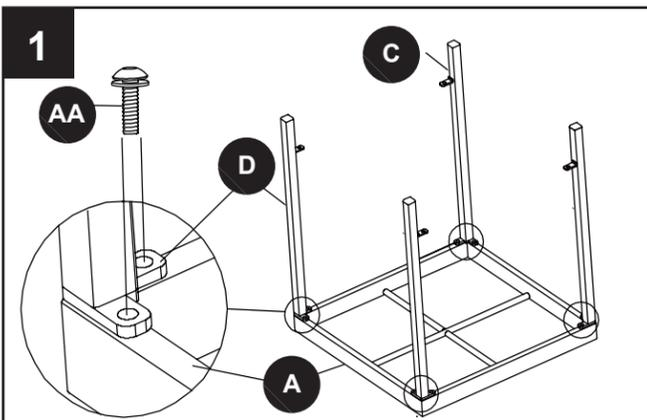
Once all connections are made, hand-tighten AA.
