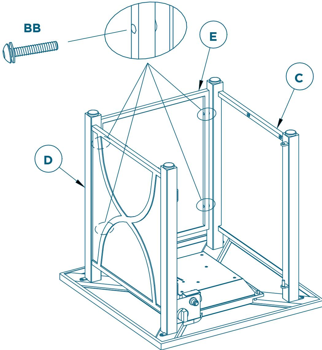
**NOTE: Do not completely tighten until all assembly is completed.**
