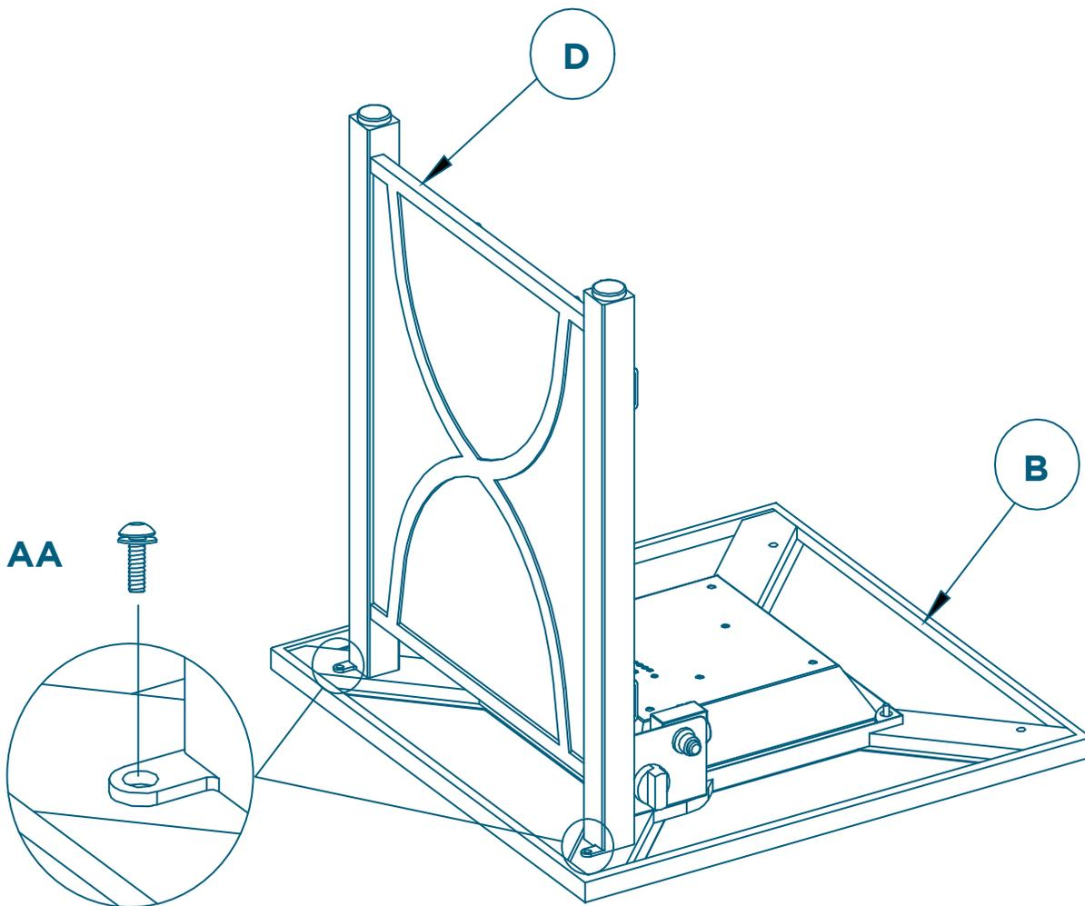
**NOTE: Do not completely tighten until all assembly is completed.**
