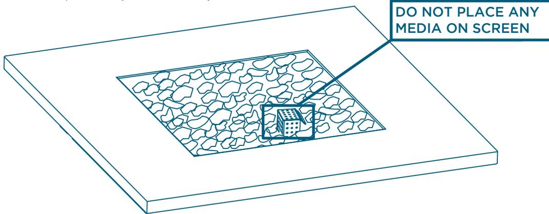
4. **IMPORTANT:** Do not exceed a height of 1" (2.5 cm) above the burner when placing lava rocks or other media. Ensure no media covers the igniter screen. Store any excess lava rocks in a safe location.
