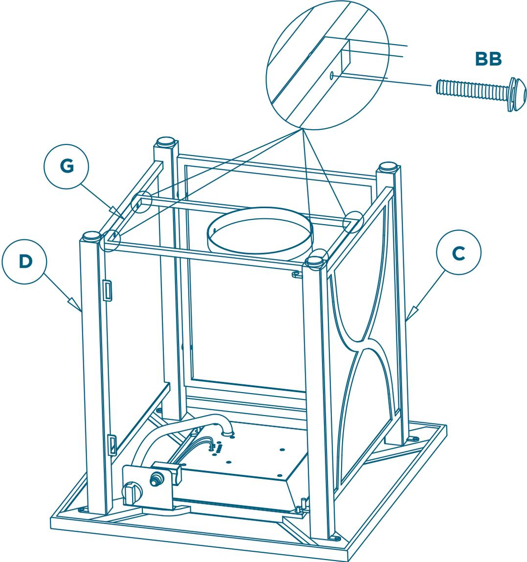
**NOTE: Do not completely tighten until all assembly is completed.**
