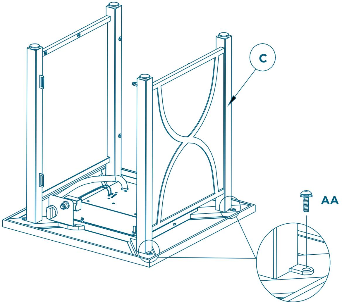
**NOTE: Do not completely tighten until all assembly is completed.**
