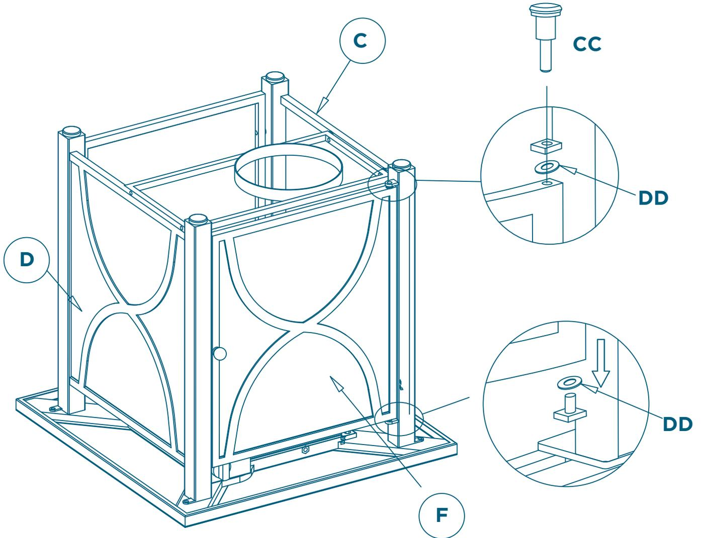
**NOTE: Do not completely tighten until all assembly is completed.**
