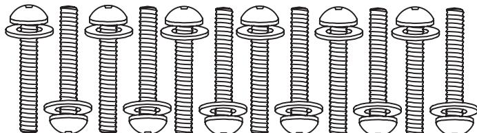
**DD** M8 x 20 Bolt (x 4) & M8 Washer (x 4)
