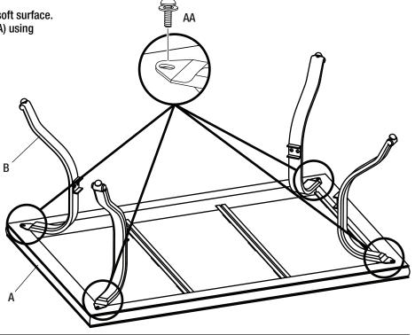
**2** Attaching The Leg Connector To The Table Legs
