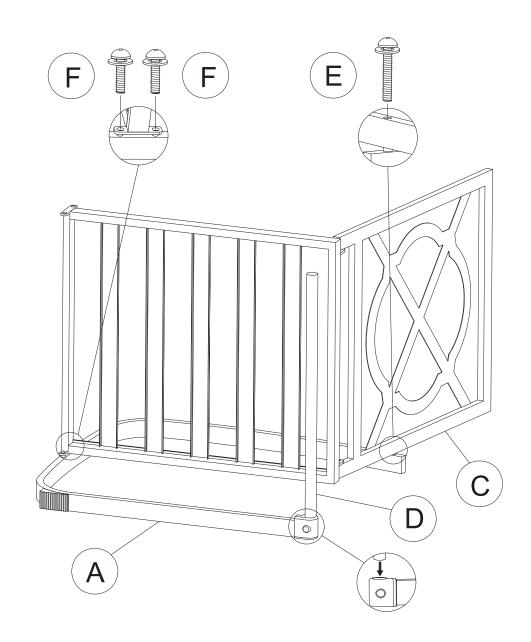
Do not completely tighten screws until all screws are in place.
