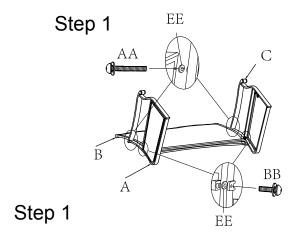
Step 1: Place the back (B) on a soft surface. Attach the left arm (C) to the back (B) by lining up bolt holes on left arm (C) with the corresponding bolt holes on the back (B). Insert M6x55 bolts with washer (AA) with plastic washers-2 (EE) as well as M6x25 bolts with washer (BB). Loosely tighten the bolts with allen wrench (FF). Repeat this step to the right arm (A) and back (B).
