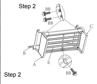
Step 2: Attach the seat (E) to the arms (A&C) and the back (B) by lining up bolt holes on the back (B) with the corresponding bolt holes on the arms (A&C). Insert M6x25 bolts with washer (BB). Loosely tighten the bolts with the allen wrench (FF). Do not completely tighten.
