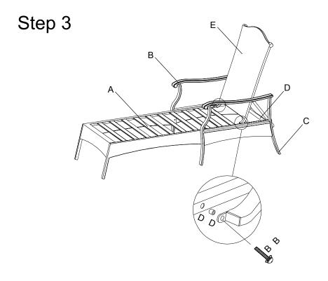
Step 3: Secure back frame (E) to seat frame (A) by lining up bolt holes on back frame (E) with corresponding bolt holes on seat frame (A). Inset M6x30 bolt with washer (BB), plastic washer - 1 (DD) and tighten using allen wrench (FF). Do not over tighten.
