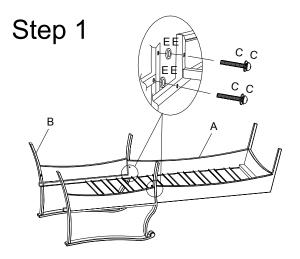
Step 1: Place the seat frame (A) upside down on a soft surface. Attach the right arm (B) to the seat frame (A) by lining up bolt holes. Insert M6x35 bolt with washer (CC) with plastic washer - 2 (EE), and loosely tighten using allen wrench (FF). Do not over tighten. Attach the left arm (C) as the above steps.
