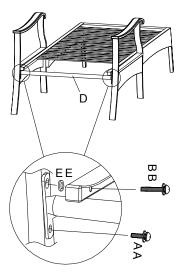
Step 2: Place cross bar (D) between right arm (B) and seat frame (A). Line up bolt holes on cross bar (D) with corresponding bolt hole of right arm (B). Secure M6x20 bolt with washer (AA) using allen wrench (FF) to tighten. Insert M6x30 bolt with washer (BB) with plastic washer -2 (EE) using allen wrench (FF) to tighten seat frame (A) and right arm (B). Do not over tighten.
