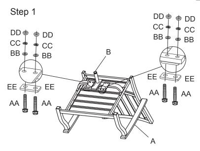
Step 1: Place the back & seat (A) upside down on a soft surface. Attach the T - R (B) to the seat support bar with M8x40 Hex bolt & washer (AA), spring metal (EE), washer (BB), spring washer (CC), and nut (DD). Loosely tighten with the Wrench (FF).
